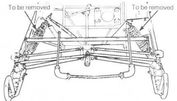
**NOTE:** If springs and dampers are changed, refer to Owner's Manual for correct front end adjustment procedure.
