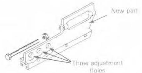
○ **NOTE:** When installing the new arm supports, use the old runner as a template. Drill the holes using a no. 13 drill bit and install new spiral pins (P/N 372 009 200).
