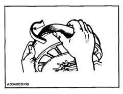
Slip the belt out from the drive pulley and remove completely from vehicle.
