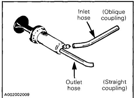
5. Plug inlet primer hose to prevent gasoline from draining.
