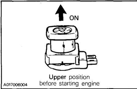
Ensure the tether cut-out cap is in position and that the cord is attached to the clothing.
