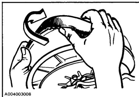
5. Slip the belt out from the drive pulley and remove completely from vehicle.
