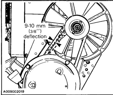
If belt seems damaged or if tension is incorrect, contact the dealer immediately.
