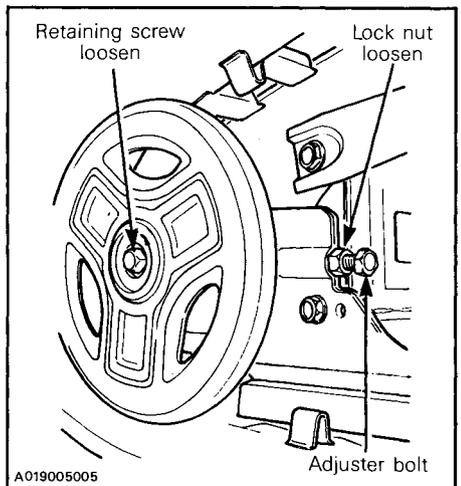
**NOTE:** Track tension and alignment are inter-related. Do not adjust one without the other.
