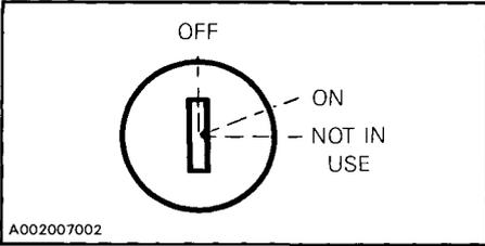
Key operated, 3 position switch. To start the engine, first turn the key clockwise to ON position. To stop the engine, turn the key counter-clockwise to OFF position.
