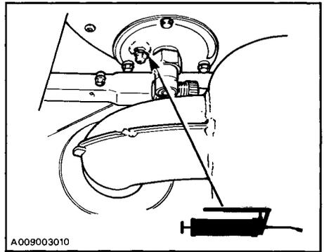
**CAUTION:** When lubricating the drive axle bearing, do not apply excessive grease as the seal will be pushed out of its housing. Check seal position with finger.
