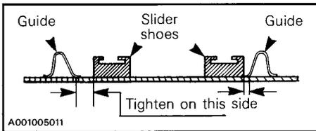
Tighten lock nuts and the idler wheel retaining screws.
