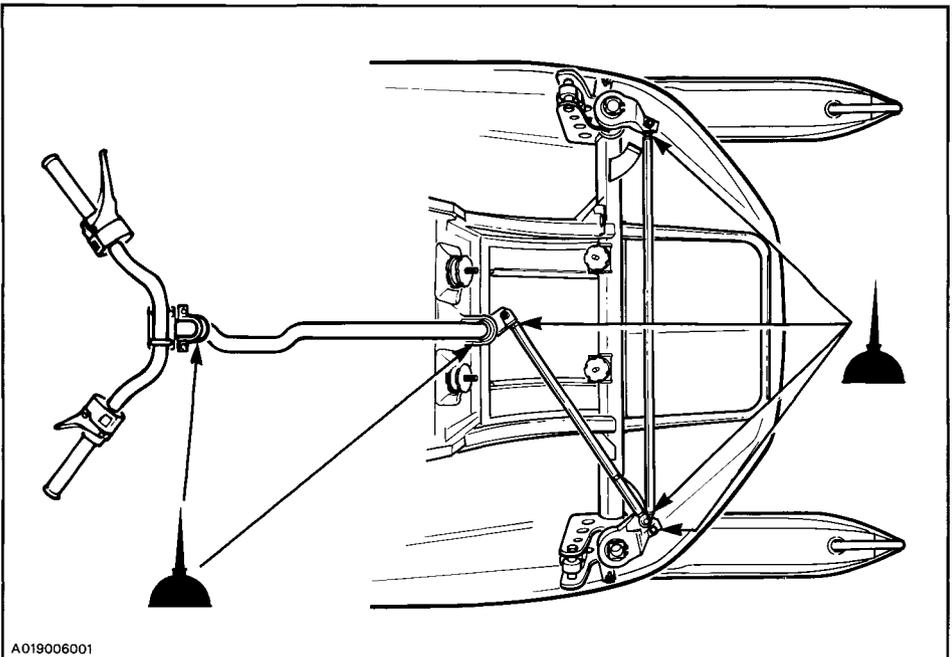
The following lubrication points have to be performed on LH & RH sides:
