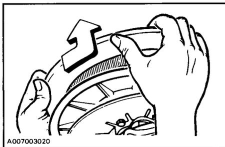
4. Slip slackened belt over the top edge of the sliding half.
