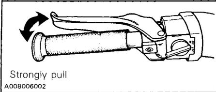
After the adjustment, brake should apply fully when lever is approximately 13 mm (1/2") from handlebar grip. If not, do not tamper with the brake, contact the dealer.
