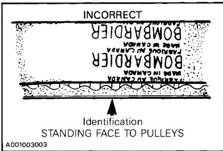
**CAUTION:** Do not force or use tools to pry the belt into place, as this could cut or break the cords in the belt.
