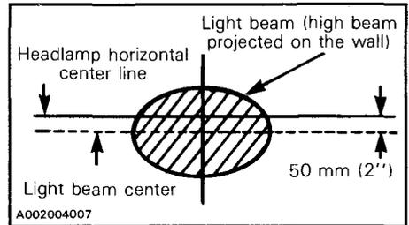
To adjust, remove the four caps, turn upper or lower adjusting screws to obtain desired beam position.
