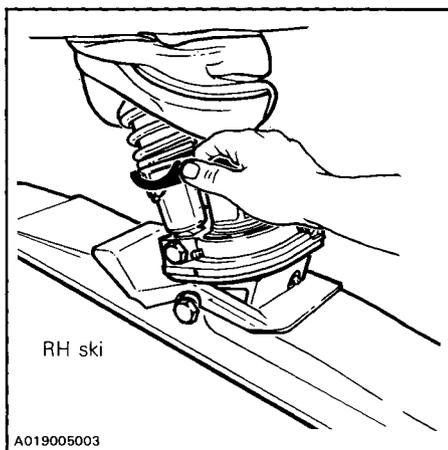
Reinstall boot and secure the spring.
