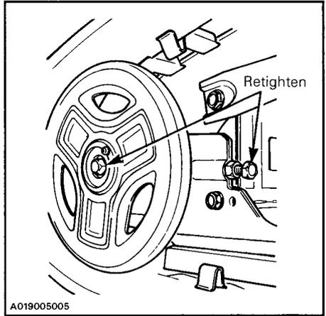
Restart engine, rotate track **slowly** and recheck alignment.
