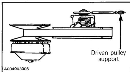
3. Open the driven pulley by twisting and pushing the sliding half. Hold in fully open position.
