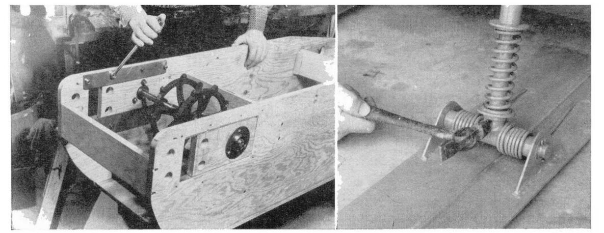
Rear sprocket bearings mount in sliding plywood blocks so they can be adjusted to stretch the crawler track taut. The blocks are held in place by strips of %"-thick steel screwed along the edges of the cutouts in the sides to form retaining flanges. Shock cord is looped through holes in the blocks and holes in the sides to pull the crawler track up tight.
