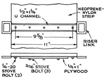
Crawler track consists of a continuous strip of neoprene-impregnated nylon belting running between U-channel crossbars. The belting is clamped to the crossbars with bolts and back-up strips of ¼" plywood, as shown above. For added strength, coat the joints with waterproof cement.
