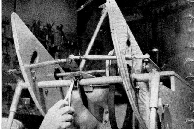
Automotive-type steering gives the Snow-Trac good control on turns. A crank arm on the central steering shaft is linked by tie rods to similar crank arms on the ski struts so that all parts move together. Note at left how the footrest boards are screwed to the side frames from the inside and are notched at the front ends to receive the curved-plywood cowl piece.
